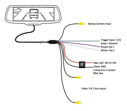
NOTE: In vehicles with LED type tail lights you may not have enough current to operate a camera or other device by drawing power from the tail lamp directly. In this case use the white tail light power as a trigger for a relay and supply power to the monitor/camera/trigger through the relay.
