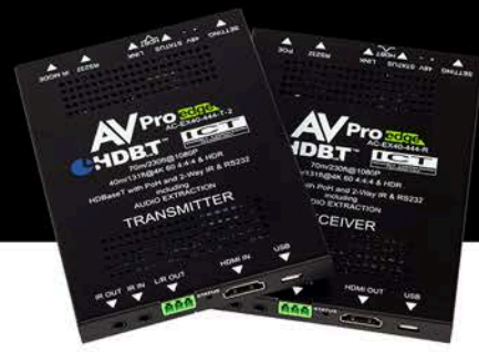
The AC-EX40-444-KIT HDBaseT point to point 40 Meter 4K Extender Kit
