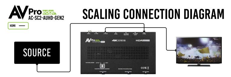
AC-SC2-AUHD-GEN2 CAN GIVE THE SINK ANY RESOLUTION FROM 480P TO 4K60 NO MATTER WHAT THE SOURCE IS OUTPUTTING
