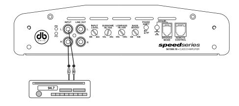
SIGNAL CONNECTION: 4 Channel Amplifier using 2 pair of RCA inputs.
