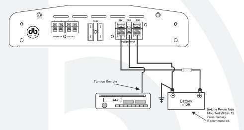
**IMPORTANT!** Before making any connections, disconnect the car's battery until the installation is completed to avoid possible damage to the electrical system.
