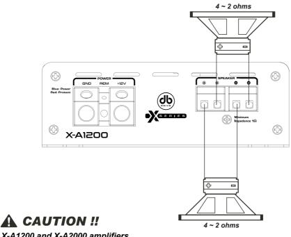
X-A1200 and X-A2000 amplifiers minimum impedance is 1 ohms.
