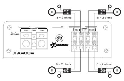
3-6B. X-SERIES 4 CHANNEL AMPLIFIERS' SPEAKER CONNECTION DIAGRAM 2.
