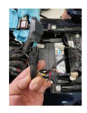
5. Plug in the Rear accessory harness and route the harness along the clutch side of the bike, alongside the factory harness.
