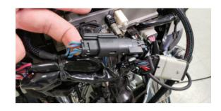
Route the harness along the clutch side to the rear pods; notice the tags for the 3. clutch side and the throttle side.
