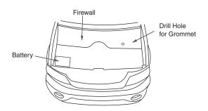
Note: To avoid any damage to parts inside engine compartment, drill from inside of vehicle using a short bit.
