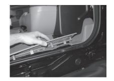
**6.** Using furnished wiring harness route 10ga red power wire starting at pre-amp location. Route wire on drivers side, over to threshold and under carpet to the front of vehicle.
