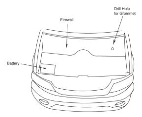
**8.** Drill a hole through the fire wall. Locate a spot low on the fire wall on the passenger side. You should always look to find a clear path. Drill a hole from inside of the vehicle into engine compartment and insert grommet. You may also find a pre-existing, unused rubber grommet in this location that you can pass the wire through.
