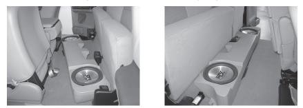
**22.** Using the supplied hardware, secure the enclosure to floor of vehicle as shown below.
