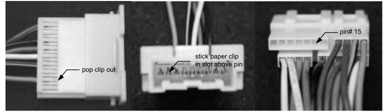
Pop white locking clip out on the OS-GM9 connector in the location of the green wire by using a small flat head screw driver.
