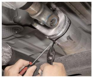
3. Using flat head screw driver and pliers crip down tie strap to secrue magnets
