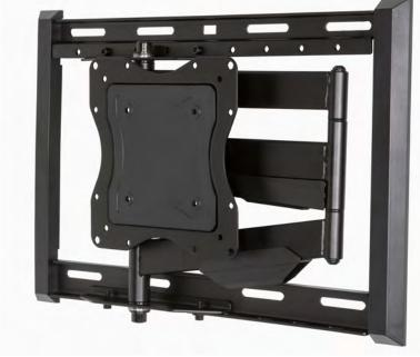
This mount allows you to have your flat panel TV either flat against the wall (2.60" low profile), tilted down for glare control or optimum viewing angle, or pulled out from the wall (21.0" extension) and angled towards a separate viewing area. With cable management, 3-way tensioning handles, and post-installation leveling, your TV will be mounted right the first time.
