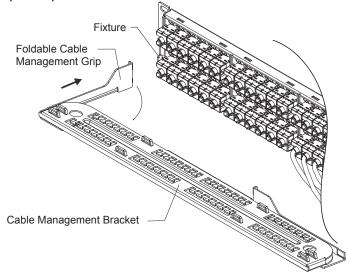
5. Fix the solid cables to the cable fixture hole using cable ties.
