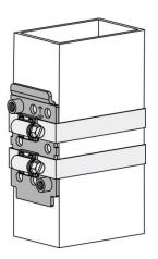
3) Use M4x8 screws to install the PVM with the VESA 75x75mm plate; and you can adjust the mounting angle/length as below by loosening the fixing screw.
