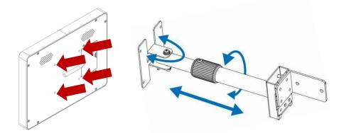
4) Attach the whole mount bracket to the plate base, and then use M6x12 screws to lock the bracket and plate base.
