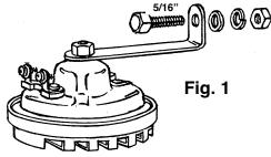
5. Attach the other end of the grounding wire to the unused horn terminal. Make sure the horn's screw terminals are securely tightened. **IMPORTANT:** Always make sure that there is an inline fuse used in the horn circuit to protect the vehicle, see chart below for correct amperage, (fuse not included). The horn installation is complete and the horn is ready to be used. Make sure wire are sure and safe.
